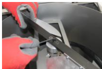
2 Loosen the central screw of the shaft.
