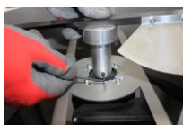
3 Tighten the screw shaft blocker
