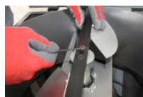
4 Tighten the central screw of the shaft.
