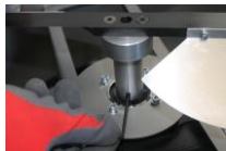
1 Loosen the lock screw shaft
