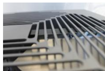
4 Close the grid and ensure that the blades don't touch the grid and they are at the desired height. (Important: keep 2mm safety distance from the grid. If not, repeat the process.)
