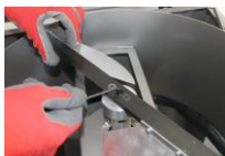
2 Loosen the central screw of the shaft.
