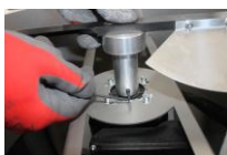
3 Tighten the screw shaft blocker
