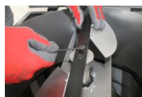
4 Tighten the central screw of the shaft.
