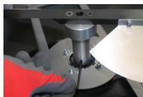
1 Loosen the lock screw shaft
